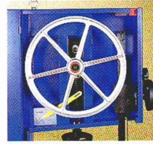
● Precisely balanced spoke design wheel ● Blade tension indicator
