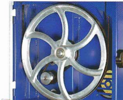
Non-Slip groove belt for smooth operation
