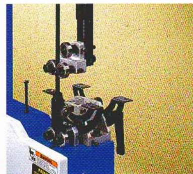
Upper and lower ball bearing blade guide system
