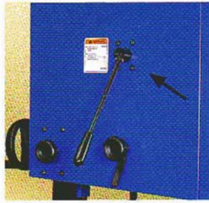
User friendly quick-release saw blade changing system
