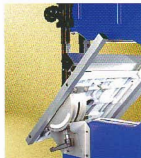
Heavy table tilting adjustment mechanism
