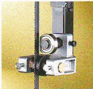
Upper and lower blade guide system
