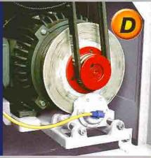
with standard. When have danger in operate main roller, can control motor stoppage in (1.5 seconds). Have sheer protective safety in operate.
